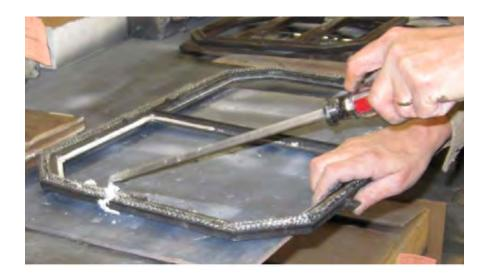
8. Apply a small bead of gasket glue to the frame and install the gasket. Use a putty knife of flat-blade screwdriver to help seat the gasket into the gasket channel. Do not allow the glue to dry before the gasket is in place or it will become hard and lumpy.
