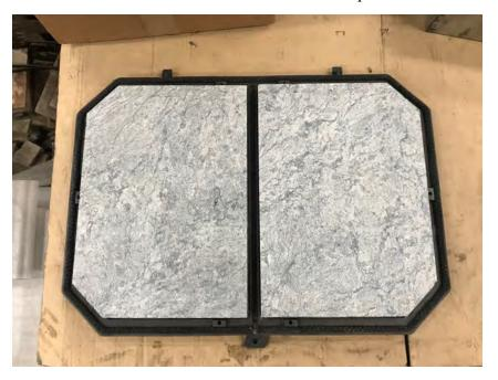
10. If the stone rests on the cast iron not the gasket, use a sander or flat file to remove stock from the edge of the two areas indicated in the following photo. Only remove enough to ensure a good fit (Maximum of 1/16")
