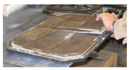
7. We recommend replacing the stone gasket at this time. Remove the gasket that rests under the stone(s). Use a putty knife or flat blade screwdriver to clean the residue from the frame as much as possible.
