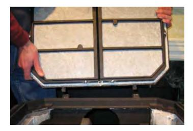
3. Place the top lid upside down on a workbench with a piece of cardboard underneath it to protect the bench and the lid.
